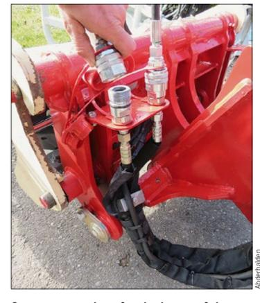
Screw connections for the hoses of the attachment can always be coupled, but it is cumbersome. Pressure relief by means of a switch in the cabin makes it easier to connect the hoses.
