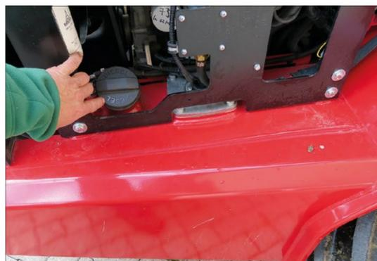
The diesel and oil tanks are fitted to the left and right in the rear part of the chassis.
