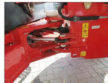
The articulated joint is new and has larger, maintenance-free pivot bearings.
