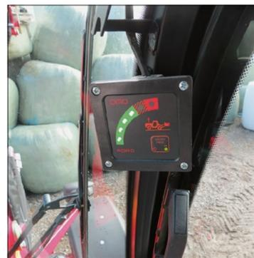
A load indicator indicates to the driver that there is no load on the rear axle is but does not actively intervene.
