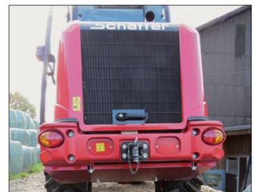
As additional weight a 200 kg plate is fitted under the rear end. The light unit is fitted in such a way that it is very well-protected.
