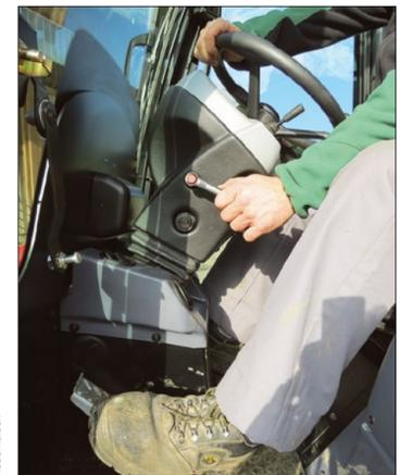
The height-adjustable steering wheel can be easily adjusted.
