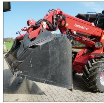
The rapid coupler holder is extremely robust and the hydraulic interlock is top notch. Practical detail: Schäffer devices have two upper coupling points. This enables a larger tipping angle whenever it is required. Another detail: The Schäffer holder is compatible with the Kramer Allrad holder.
