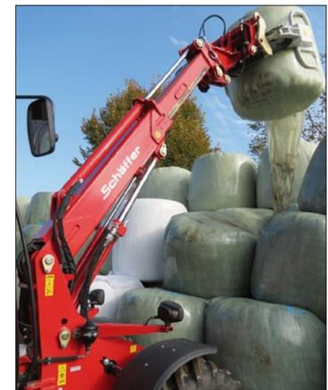
Solid telescopic arm with 100 cm and Z kinematics. The hydraulic parallel guide tool adapts the angle of the attachment to the loading system using Z kinematics.
